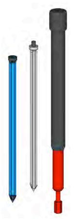
Insert the pilot rod only as far as needed for the length of probe being used. A hole that is too short may cause damage to the probe during insertion. A hole that is too long may allow water to collect in the void below the probe and cause inaccurate readings.
