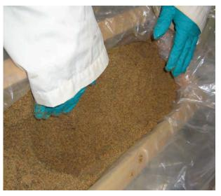
Push the sampling ring into undisturbed soil on the side of the hole. Try to ensure no additional soil compaction, that is do not pack the cylinder more tightly or less tightly than the surrounding soil (this will introduce an error in the sample.
