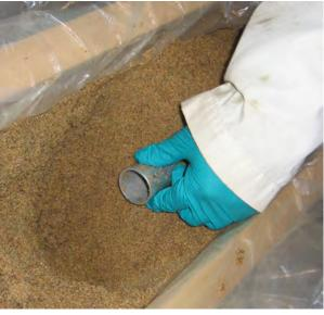
Remove the sampling ring from the soil by scraping the surrounding soil away (use the tongue depressor) until the ring is exposed.
