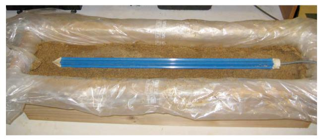
**Soil container/box** – must be of sufficient volume to contain enough soil to extend at least 7-8 cm around the probe in all directions. If necessary, a container may be made from wood, if so, then it should be lined with heavy plastic sheeting to prevent any loss of moisture due to drainage or absorption by the wood. The above example box is a commercially available wooden planter box, approximate <u>inner</u> dimensions 7.25" high by 7.5" wide
