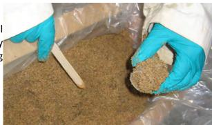
Cut away any excess soil from the open ends of the sampling ring, and also ensure the that the outside of the sampling ring is free of soil.
